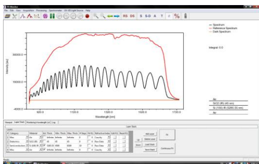
Figure 1: Typical reflectance spectrum for a suspended Si(100) membrane on an ultra thin SiO 2 layer.
